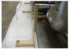
Safeguarding by means of wood/wedges
