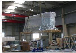
Weighing of the finished package
