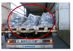
Incorrect securing of the load, not enough lashing straps
