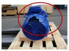
Damage due to incorrect securing of the load / missing outer packaging
