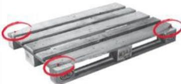
More than two bottom or top edge boards have splintered in such a way that, in total, more than one nail or screw shaft is visible.
