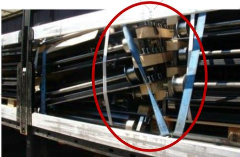
Incorrect securing of the load, lashing straps not positioned correctly
