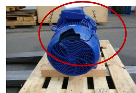
Damage due to incorrect securing of the load / missing outer packaging
