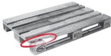
A bottom or top edge board has splintered in such a way that more than one nail or screw shaft is visible.
