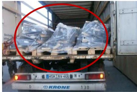
Incorrect securing of the load, not enough lashing straps
