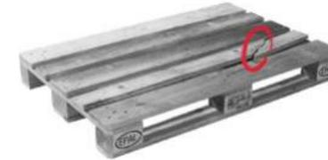
A board is broken transversely or diagonally.
