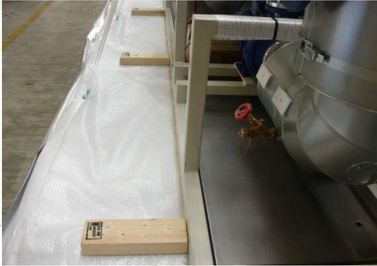
Safeguarding by means of wood/wedges
