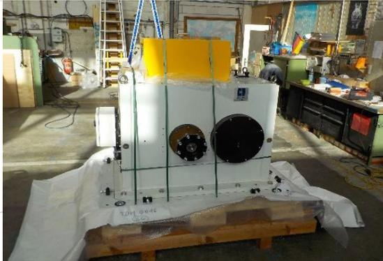
Secure the machine on the bottom of the case
