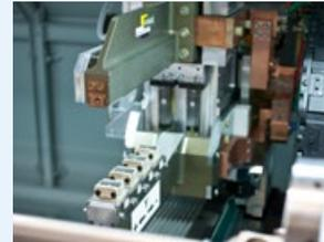
Fully automatic quadropole weld electrode
