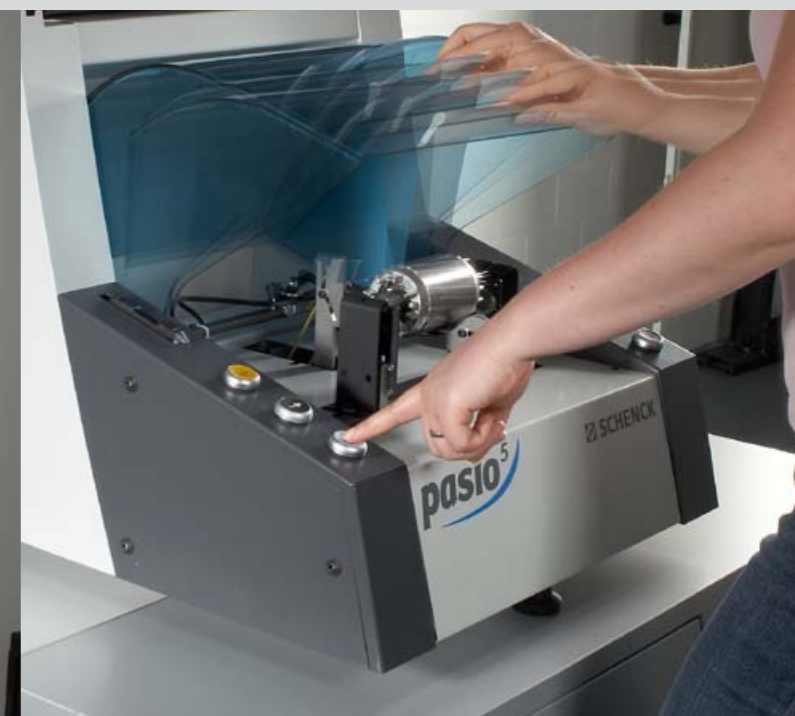
Protective cover for rotors with sharp-edged surfaces
