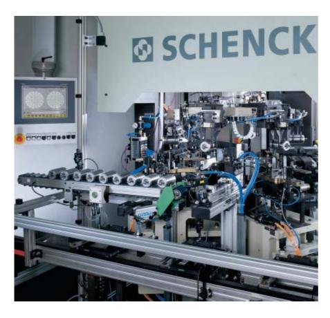
Integrated overhead rotary transfer machine
