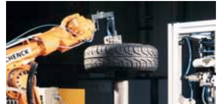
Automatic application of adhesive weights
