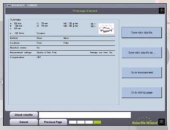
Saving rotor data and starting the measuring run.
