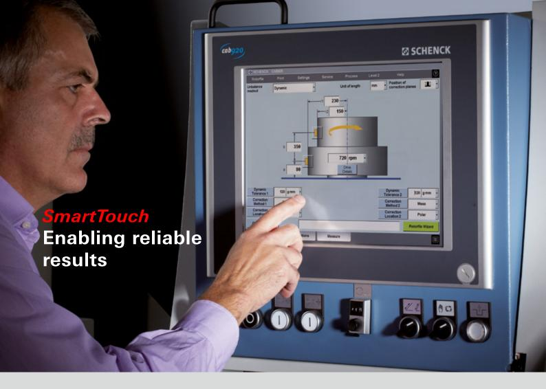
Smart Touch is the name of the intuitive user interface. All information for the balancing procedure is clearly combined and called up through three tabs. Depending on your balancing experience, two navigation methods are easily accessible.
