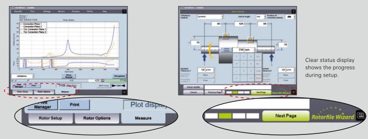
3-tab navigation field for fast and direct access to all functions.
