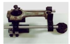
Plane calculation and classification: As above, however with separate indication of up to 20 classes, after recalcuation to the bore center of the conrod for measurement in arbitrary planes
