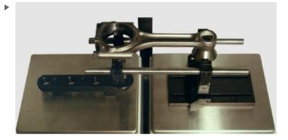
Adapter frame for unmachined conrods, also adjustable for different sizes. Suitable for production checks in forges and foundries as well as for receiving inspection.
